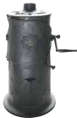
1879 Ball or spheric roaster first generation AZ 3kg per batch.
